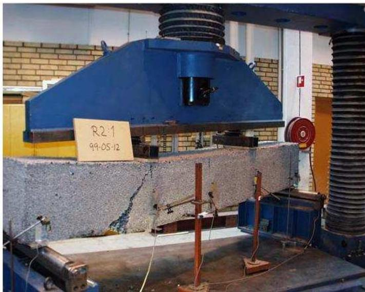
*Figure 4.5 Full scale testing of LLP*
