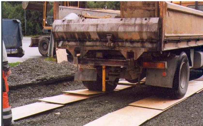
*Figure 4.12 Plate loading test directly on LWA layer*
