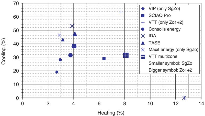
Figure 6. Relative difference in the needs for annual heating and cooling energy between the extra-light and the massive single-family houses using various simulation programs and single-zone and double-zone models.
