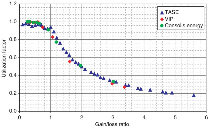
Figure 12. Monthly gain utilization factor for the massive single-zone, single-family house according to TASE, VIP and Consolis Energy.
