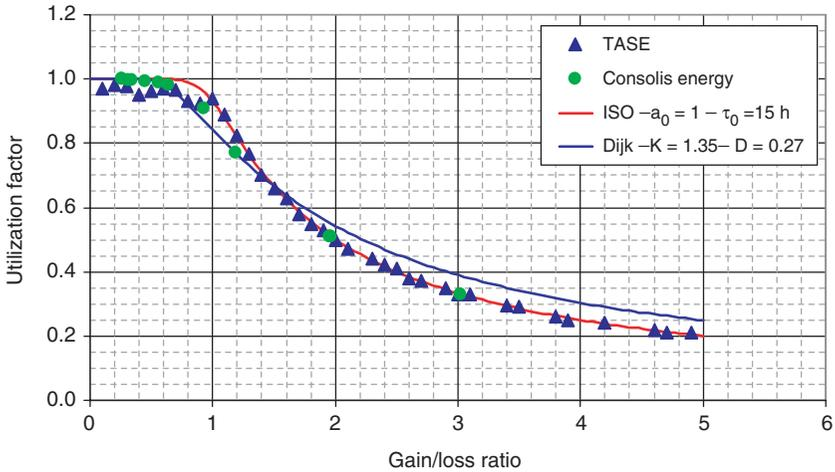
**Figure 15.** Monthly gain utilization factor for the massive single-zone, single-family house according to TASE, Consolis Energy, ISO DIS 13790 and van Dijk and Arkesteijn.
