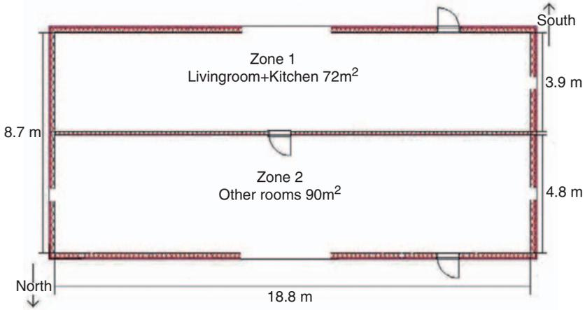
**Figure 1.** Single-family house modeled using two zones. Main facades in east–west direction.
