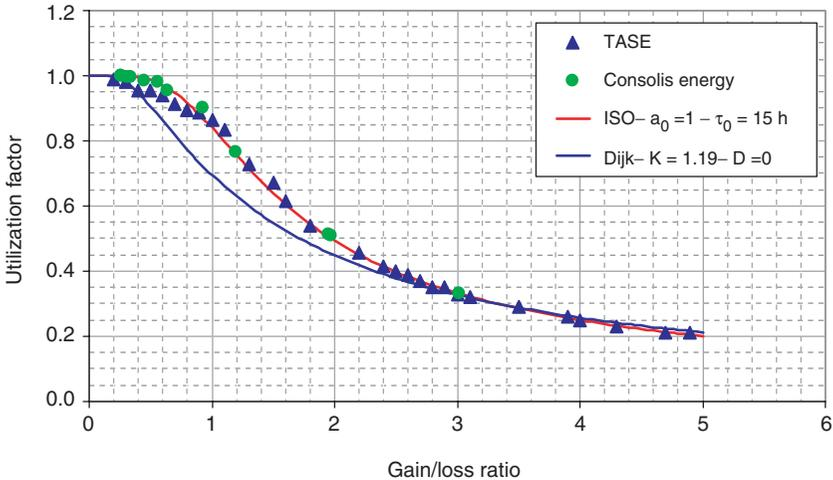
**Figure 14.** Monthly gain utilization factor for the light single-zone, single-family house according to TASE, Consolis Energy, ISO DIS 13790 and van Dijk and Arkesteijn.
