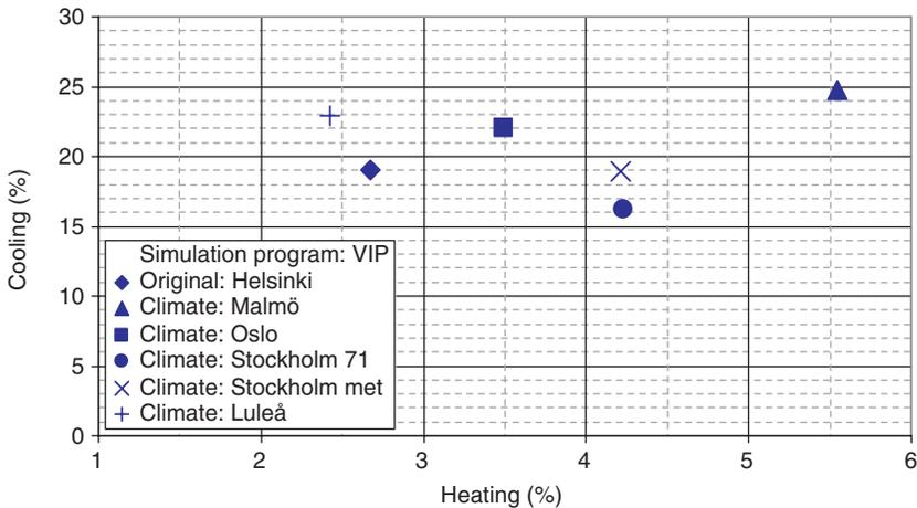
**Figure 9.** Effects of weather data used and thermal mass on the relative difference between the needs for annual heating and cooling energy of the extra-light and the massive single-family houses. Single-zone building. Calculations made by VIP.
