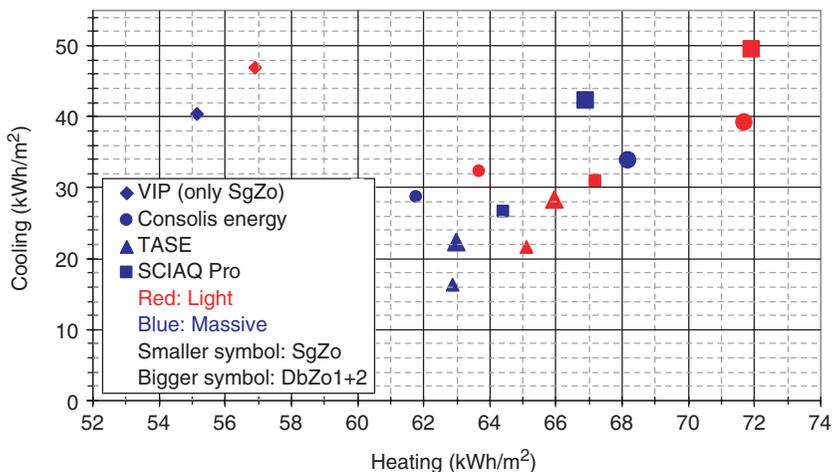
**Figure 4.** Annual heating and cooling energy for the apartment flat. Single-zone (SgZo) and double-zone (Zo1+2) cases.
