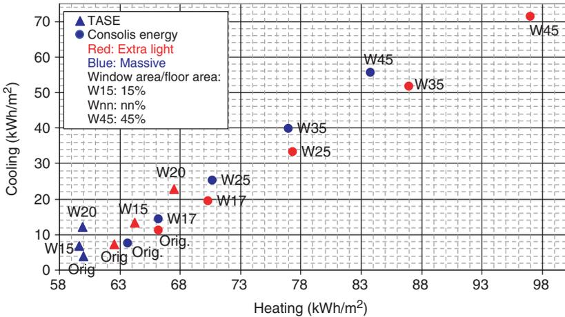
Figure 7. Effect of windows' orientation and size on the annual heating and cooling energy. Double-zone, single-family house.
