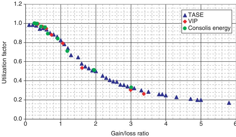
Figure 11. Monthly gain utilization factor for the extra-light single-zone, single-family house according to TASE, VIP and Consolis Energy.
