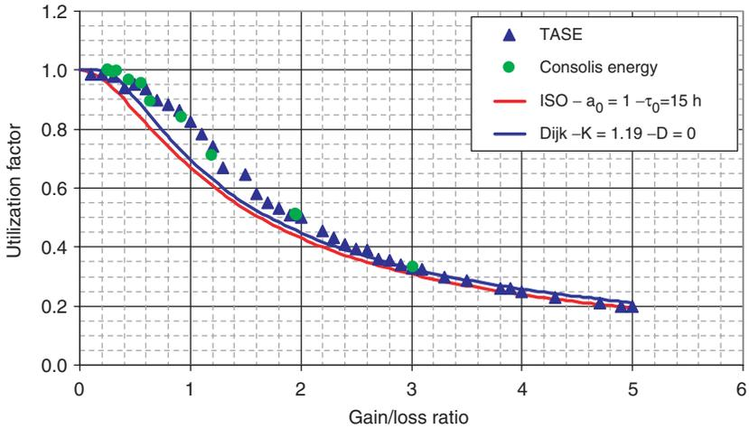
**Figure 13.** Monthly gain utilization factor for the extra-light single-zone, single-family house according to TASE, Consolis Energy, ISO DIS 13790 and van Dijk and Arkesteijn.
