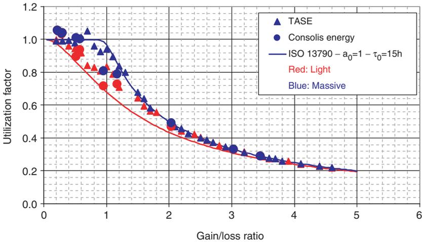
**Figure 16.** Monthly gain utilization factor for the extra-light and for the massive double-zone apartment flat according to TASE, Consolis Energy and ISO DIS 13790.
