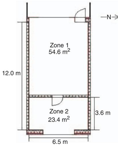
**Figure 2.** Two-roomed flat of the apartment building. Facades in north-south direction.
