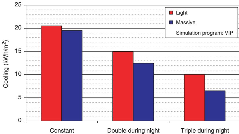
**Figure 10.** Effect of night-ventilation and thermal mass on the annual cooling energy. Apartment flat. Calculations made by VIP.
