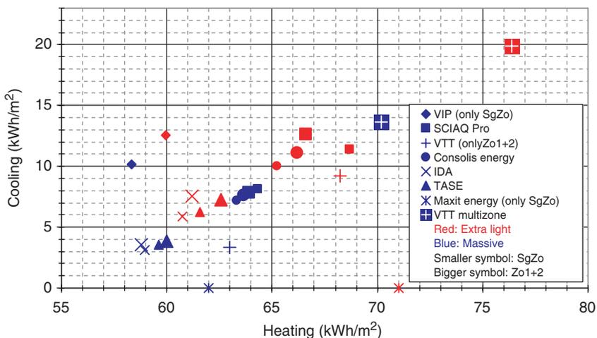
**Figure 3. Annual heating and cooling energy for the basic case of the single-family house. Single-zone (SgZo), double-zone (Zo1+2), and 15-zone (MulZone) cases. Maxit energy calculates only heating energy.**
