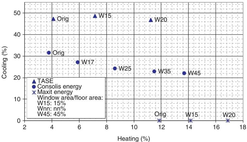
Figure 8. Effect of windows' size on the relative difference between the needs for annual heating and cooling energy of the extra-light and the massive single-family houses. Single-zone building in maxit energy, in others double-zone building. Basic window area 12% from the floor area.
