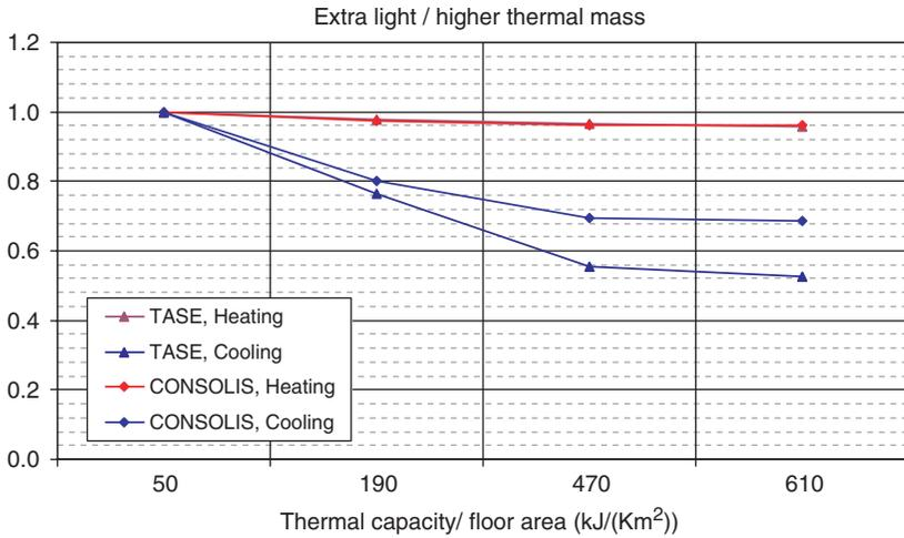
Figure 5. Effect of thermal mass on the annual heating and cooling energy. Single-family house, a double-zone model.
